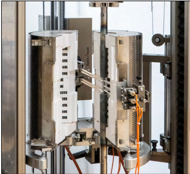
makroXtens II 100 HP on high-temperature furnace HTF-LVW 1,250 °C
