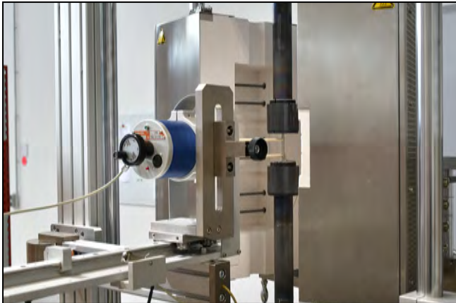
High-temperature contact extensometer up to 1,500 °C
