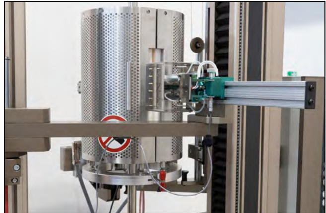
High-temperature contact extensometer up to 1,600 °C
