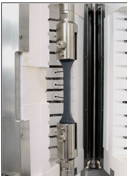
II) High-temperature specimen adapter for shoulder-end specimens with hole and fixed thermocouples (attached)
