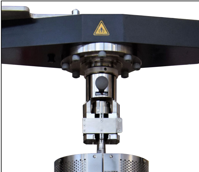
Load string with mounting studs and furnace
