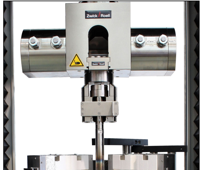
Load string with T-slotted shoe connector and furnace
